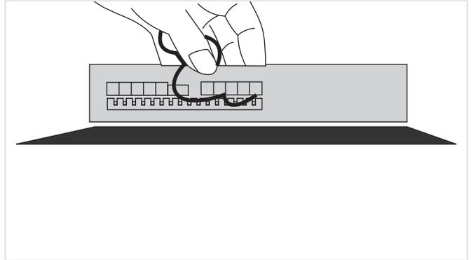
Strip off 10 mm (approx 1 cm ) of the load wire ends that are to be connected. Note that excess stripping will lead to shorts between two wires. Connect the load wires as per the stickers mentioned on the box. Ensure that there are no wire strands protruding outside the connectors.
