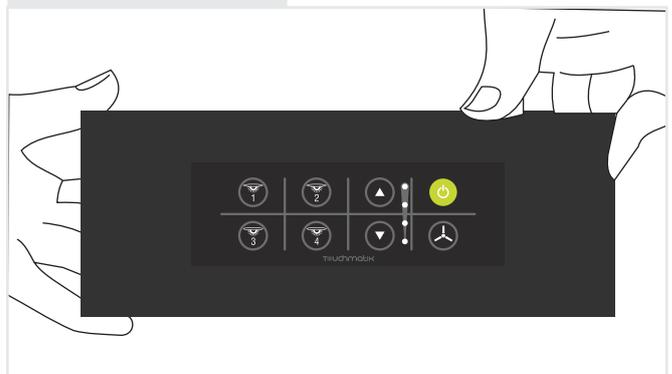
Ensure proper fitment of the switch board vertically and horizontally. Check the whole switch board functionally. Check the switch board for Remote operation if applicable.
