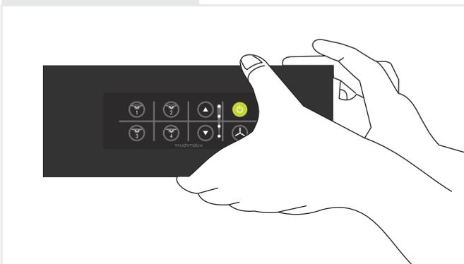
Check the whole assembly by switching on the loads one by one. Press Fit the top black cover plate to the switch board.
