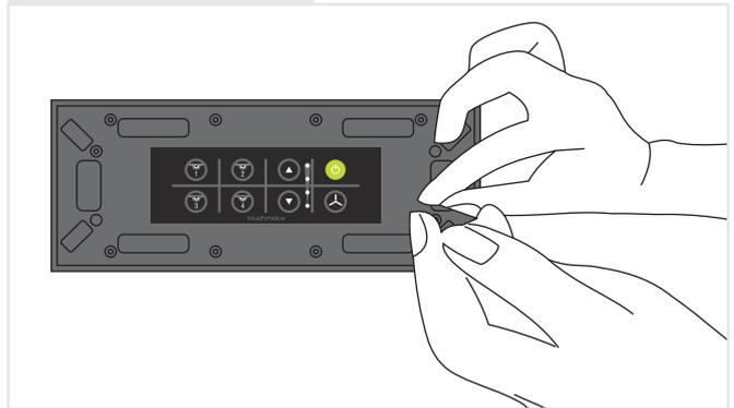
Screw fit the switch board to the conceal box (use the screws provided along with the switch board). Ensure that there is no stress on the load wire connections and the box fitment.
