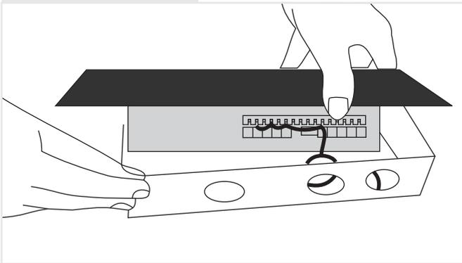
Align the loose cables in the concealed box properly. Place the switch board over the conceal box.
